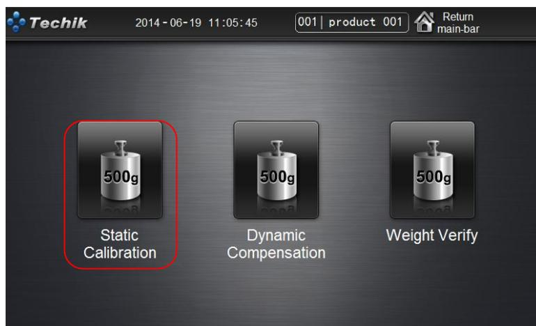
Please press "1..zero calib" button in the bar of "Static Calibration" and operate according to notice.
