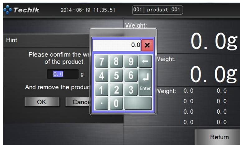
You can directly apply the product weight value in the input box which already existed, or manually type in the correct product weight value. Press "OK", the conveyor belt starts to run, and then "Dynamic Compensation" starts. Please put product on the input side of belt to proceed dynamic weighing.
