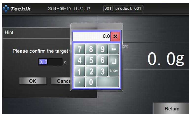
Type the real value of the weight in the pop-up input box, and then press "OK" to proceed the operation of "fixed points calib". The "Static Calibration" operation will succeed after the notice, Press "Return" to return back to "Machine Calib" bar.
