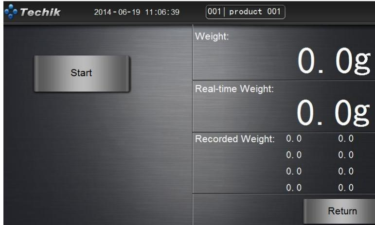
Attention: "Dynamic Calibration" requires products pass the check weigher at least 8 times, pls make sure the dynamic weighing value fluctuation is not too big in "recorded weight".
