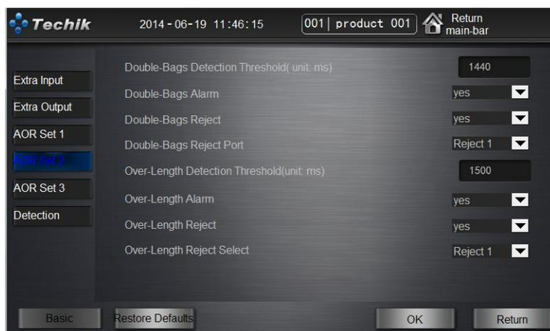
"Double-Bags Abnormal" refers to the weighing error situation caused by the too short time period between each two products(also means too short distance between each two products).
