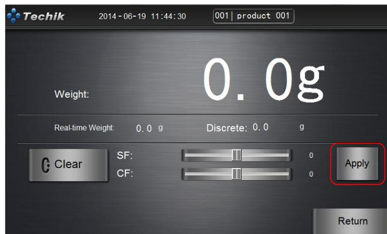
You can see the dynamic weighing result after product proceeding "Dynamic Compensation" in "Weight Verify" bar. If you have got the weighing result and then no need for you to adjust in "Dynamic Verify" bar.
