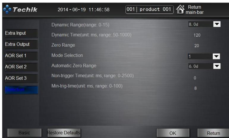
"Dynamic Range", "Dynamic Time" and "Dynamic Time" are mainly on the special condition without light and electricity detection application.
