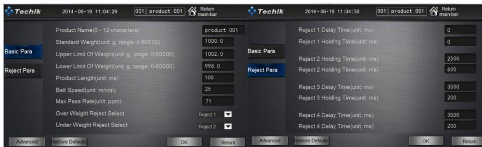
After setting the parameters of the product, click on the "OK" button to confirm the parameter download. If you want to give up this parameter setting, click "Return" to return to the "Product editor bar." "Restore defaults" button can restore the parameters to the last parameter setting.
